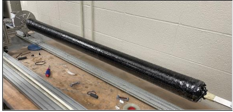
Figure 7: X-Winder Lower Airframe Tube Winding
