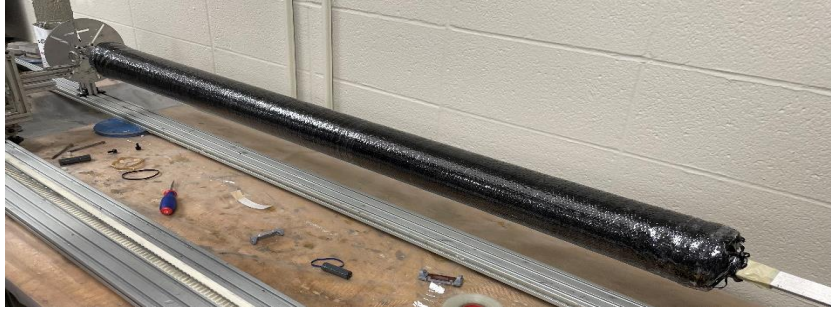
Figure 3: X-Winder Lower Airframe Tube Winding
